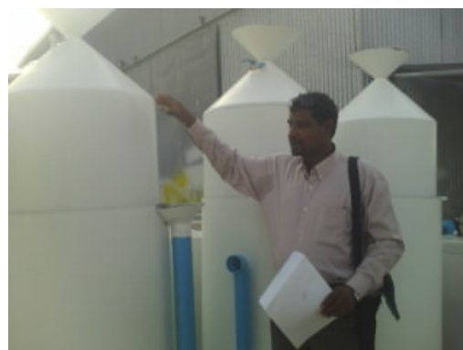
FIGURE 20: Bio-digester plant manufactured by GFF in Thilafushi
