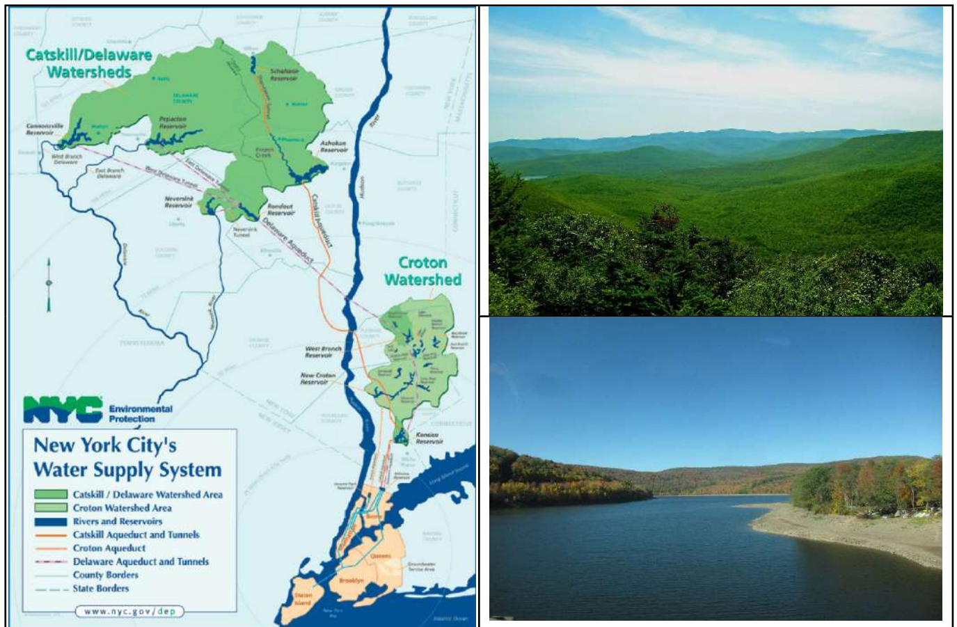
Figure 2-3: New York City's water supply system (Left above, Source: www.nyc.gov/dep ) includes 90% unfiltered water sourced from Catskill/Delaware watershed 100 miles away includes; Catskill watershed view from Twin Mountain south summit (Right above, Source: Wikipedia.org) and the Pepacton reservoir (Right bottom: Source: Wikipedia.org)
